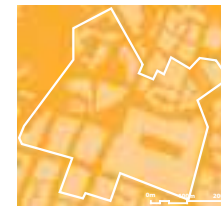
fig.75 Manchester Millennium Site Area: 20.1ha Plot Ratio: 1.4 Site Coverage: 59% Mean Number of Storeys: 4.0
