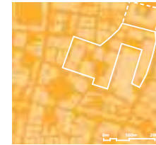
fig.72 Broadgate, London Site Area: 8.6ha Plot Ratio: 4.2 Site Coverage: 60% Mean Number of Storeys: 8.6
